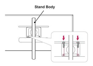
3 Insert the **stand base** into the hook of the **stand body**.
